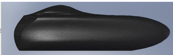
Drawing on Solidwork of the recumbent bike body
