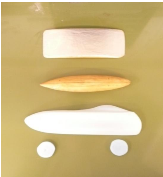
The balsa mock-up of the recumbent bike body
