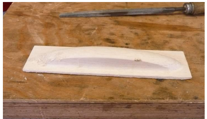
The balsa mock-up of the recumbent bike body
